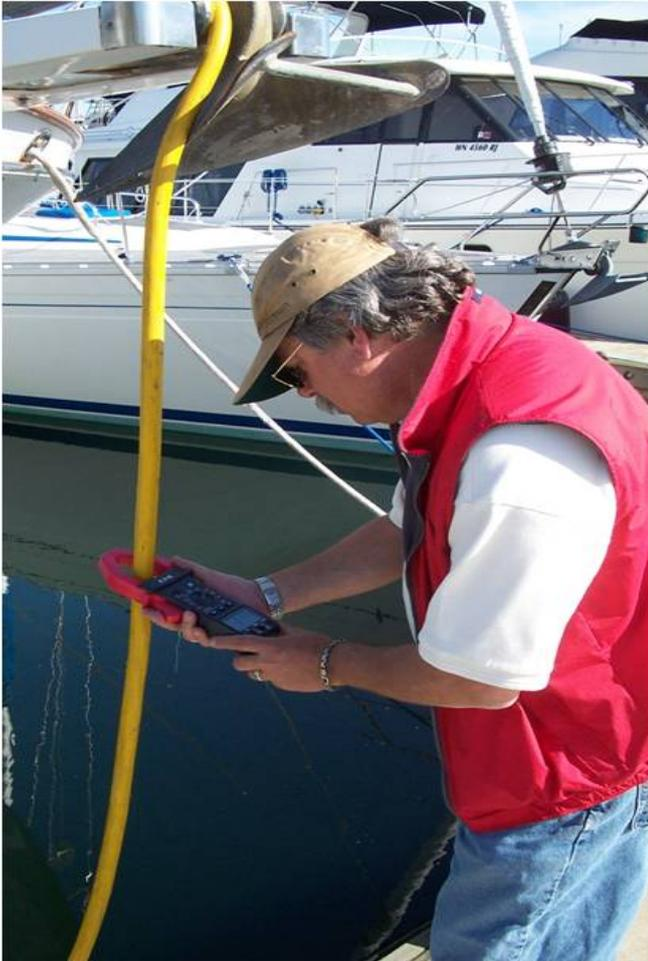
To the uninitiated the photo above shows me doing something with a clamp-on ammeter that is counter to what most folks have been taught to do with said tool. In general, when you are measuring amperage flow through a conductor you only want to clamp around one wire. In the situation above I'm clamped around the entire shore power cord to the boat in question, and there are three individual wires, or conductors inside that yellow insulation.
