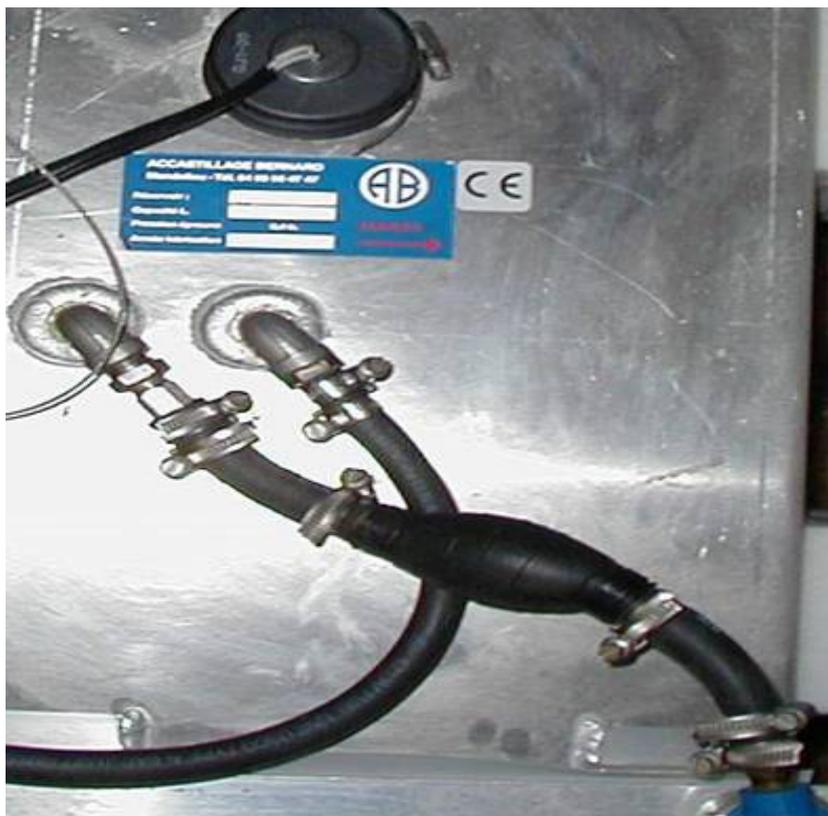
This one is easy to answer. The ABYC does NOT require that double hose clamps be used anywhere in your fuel system other than for the fuel fill hose. Double clamping of the fuel fill hose is a USCG requirement under Title 33 of the Code of Federal Regulations for recreational boats. In this case the ABYC Standards (H-24 and H-33 for gasoline and diesel systems respectively) mirror the Coast Guard requirements.
